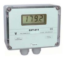
The SXT-81U transducer converts temperature from an input sensor to the output signal 0...5 mA, 0...20 mA, 4...20mA, 0...5V or 0...10V with galvanic separation between an input sensor and the output.
