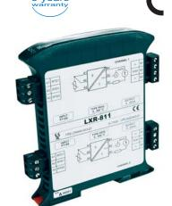
The LXR-811 transducer converts temperature from the input sensor Pt100 / Ni100 to the output signal 4...20mA. A device works as a current loop regulator with galvanic separation between the input sensor and the output. The LXR-811 is self powered from the current loop.
