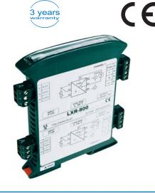
The LXR-800 temperature transducer converts temperature from the input sensor Pt100 / Ni100 to the output signal 0...20mA. Built-in, high precision resistor 500Ω allows for easy conversion current signal 0...20mA to the voltage 0...10V.
