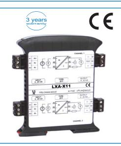
The LXA-X11 isolator is dedicated for separation analog input signal from the output line 4...20 mA. A device works as a current loop regulator with galvanic separation between input and output. The LXA-X11 is self powered from the current loop.
