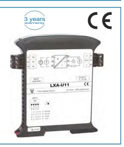
The LXA-U11 universal analog isolator is dedicated for separation an analog input signal from the output line 4...20mA. A device works as a current loop regulator with galvanic separation between input signal and output. The LXA-U11 is self powered from the current loop.
