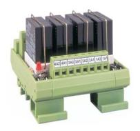
The LMP-51K-4 relay module is designed as output device for a control unit. A module consist of four independent channels. Each channel has two independent NO / NC contacts. Every relay is easy detachable thanks to the holder. Appropriate LED diode indicates relay acting. There is possibility to deliver device for non-standard coil voltages.
